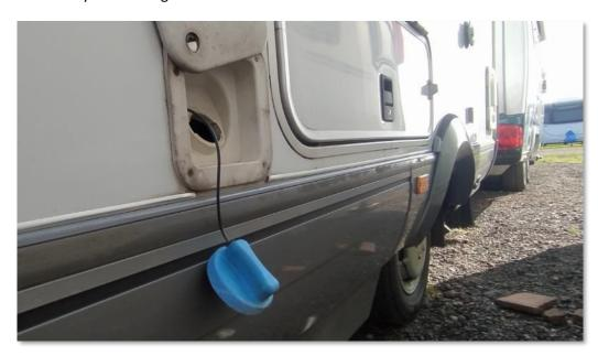
Waste water flows down the plug holes into a 'grey water' tank. This also tends to hold about 100 litres. To empty the grey tank, you'll need to drive over a suitable drain and then open a tap on the outside of the van to let the used water flow away. Or you can use a bucket if you don't want to move the van or can't get over the drain.
