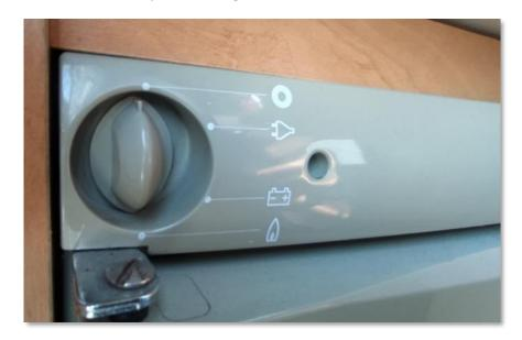
A few vans have 'compressor fridges' which work on 12 Volts when you're parked but these are relatively rare. The three-way fridges in most vans will only work on 12 Volts when your van's engine is running.
